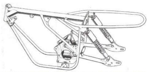
The new frame complete with rear suspension and gearbox plates; the rear fork is pivoted on those, not on the frame structure.
