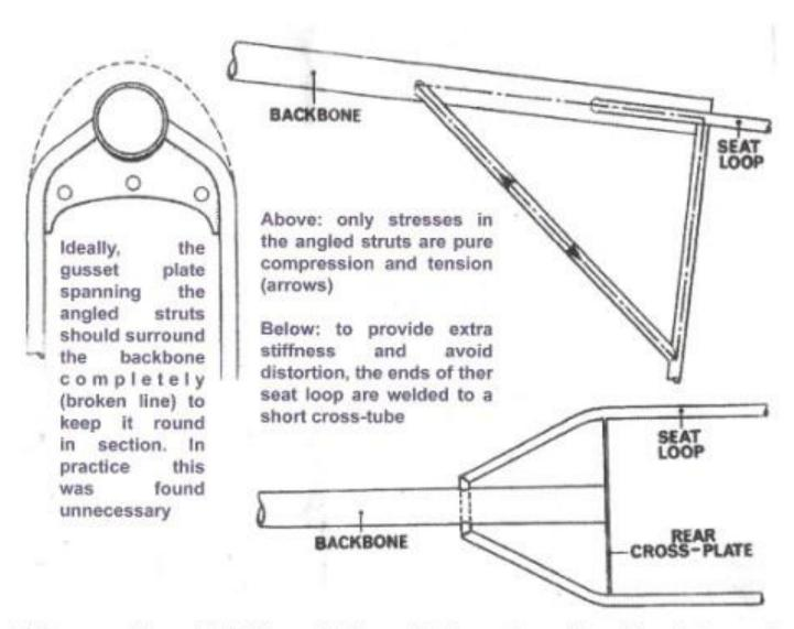
twisting moment is carried right through to the steering head.
