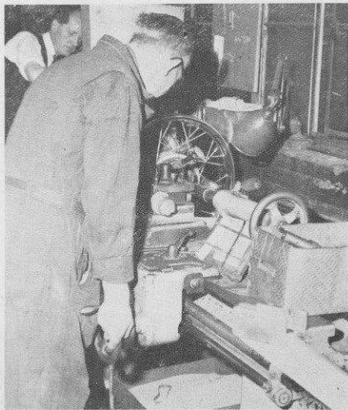
With the spokes and brakedrums in position the wheels pass on to this machine where the operator tests them for "true"
