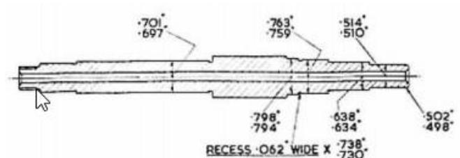
The shaft is clamped to the shoulder of the original diameter. The 0.638" and 0.763" diameters are turned simultaneously, at a rate of 695 rpm. After drilling the  $\frac{13}{64}$ " centre hole, the shaft is supported in the lathe by means of a rotating centre point. This drilling is done over a length of  $4 \frac{3}{8}$ " , at a speed of 930 rpm. And manual feed. For the other operations, the feed of the support is automatic. Duration  $4 \frac{1}{2}$  minutes.
